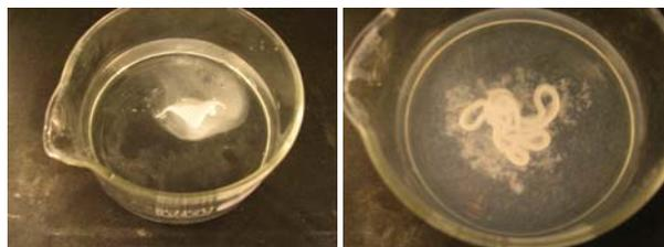
Fig. 1: Photos of calcium aluminate extruded after 3 minutes into tap water (left) and PBS (right)
